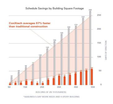
The data indicates that in either case - the higher or the larger the project - the greater the comparative schedule savings versus a traditional steel erection process. The comparative benefit is most prominent, however (by about 30% per story), as the building increases story-to-story, given the unique process advantage of the ConXtech system.
